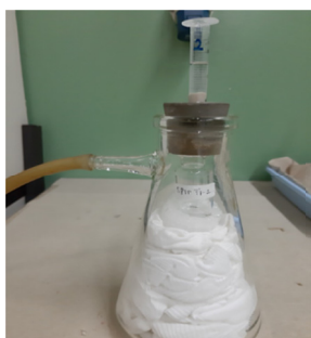
Fig. 1: The process of separating ^{137}Cs with a cation exchange column using Lampung zeolite.
