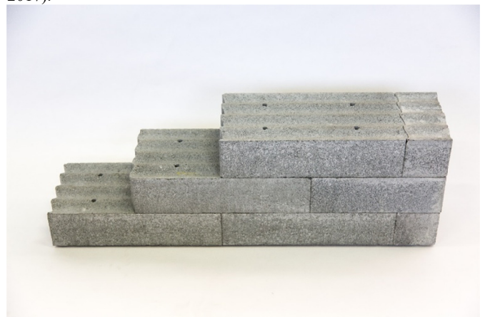
Fig. 1: Low-activity concrete bricks developed for shielding. Typical activities are ^{226}\text{Ra} \approx 0.6 \text{ Bq/kg} , ^{228}\text{Th} \approx 0.3 \text{ Bq/kg} and ^{40}\text{K} \approx 6 \text{ Bq/kg} .
